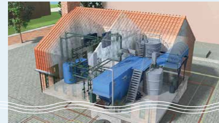
Noorderhoek, Sneek, (NL) "Waterschoon" project, local wastewater treatment for 207 houses
