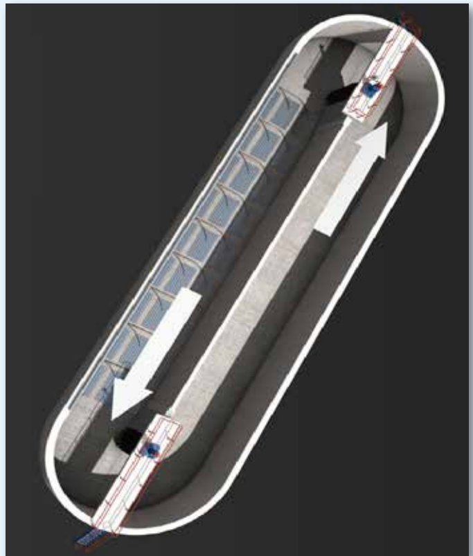
Continuous aeration grids with LANDOX flow booster
